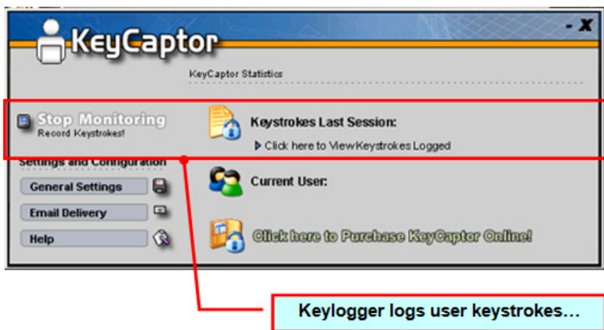
Figure 4-8: Keylogger example with user keystroke information.
